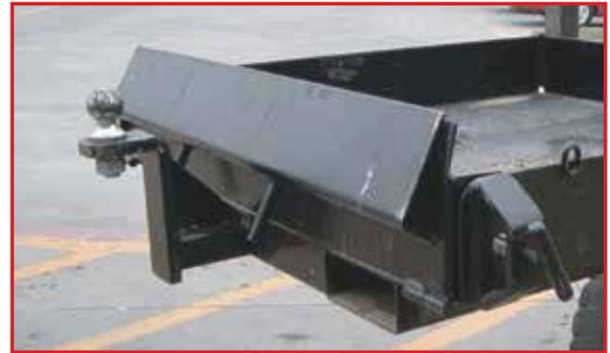
Built-in receiver for moving trailer mounted equipment. Accepts standard 2” sq. trailer adapter. (Shown with optional adapter and ball.)
