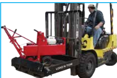
Spring loaded pin locks ramp in “up” position for secure and safe transportation of load.
