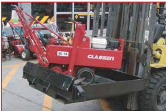
Spring loaded pin locks ramp in “up” position for secure and safe transportation of load.
