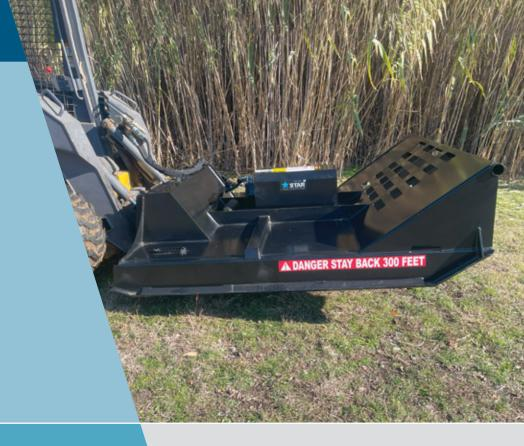
The Star Industries Skid-Steer Brush Cutter is the tough, all-terrain cutter perfect for clearing overgrowth on median strips, farm and ranch, parks and land clearing for development. The cutter is equipped with 3 versatile bi-directional blades powered by a high-torque motor and 100-hp Omni gearbox capable of powering through the toughest of terrains.
