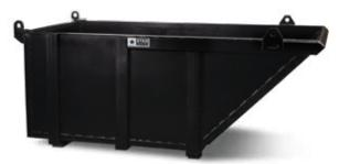
To dump the skip, the two forward slings are disconnected from the lifting eyes with the lifting line slack. The skip is then lifted with the rear slings still connected, effectively dumping the load from the sloped end.
