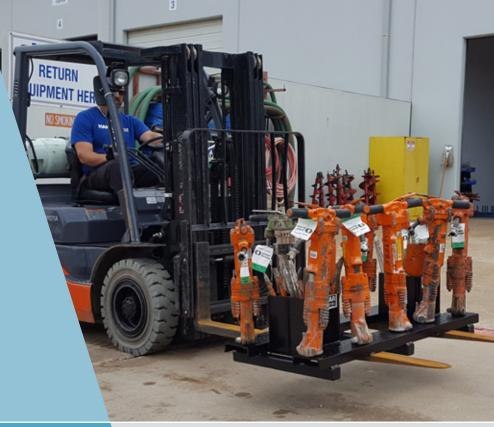
Keep your paving breakers and moil points protected and secure all in the one place with a Star Industries Paving Breaker Pallet. The Pallet can store 10 breakers and 64 moils (8 moils per cylinder).
